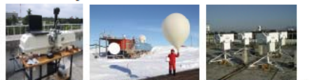
Figure 3. Ozone layer monitoring by an automated Dobson ozone spectrophotometer (left), a balloon-borne ozonesonde with an electrochemical concentration cell (ECC) (middle): at Syowa station in Antarctica, and Brewer spectrophotometers (right).
