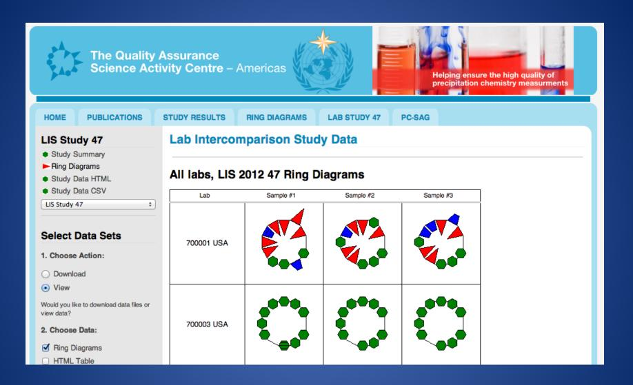
An example of two U.S. labs, one that performs well and one with some analytical problems.
