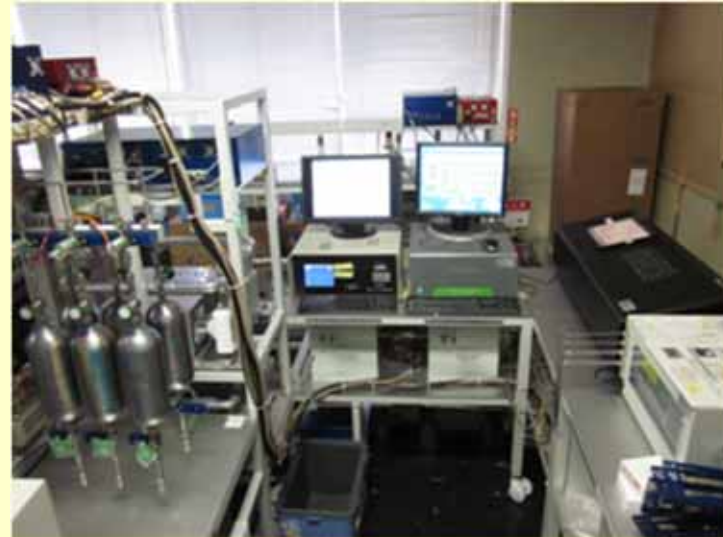
Measurement of CO 2 , CH 4 , CO, N 2 O concentrations
